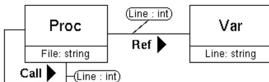
**Figure 4.** Schema (class diagram) for graphs like the one in Figure 1.
