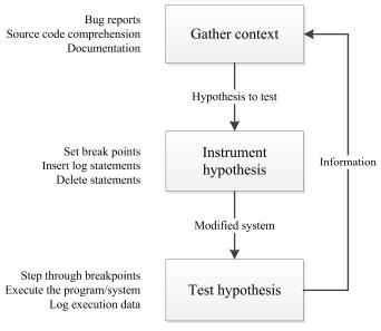
Fig. 3. Debugging process model
